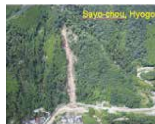
Slope failure (Typhoon No.9, 2009)
