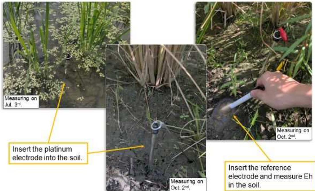
Fig.4 the measurement of oxidation-reduction potential Eh
