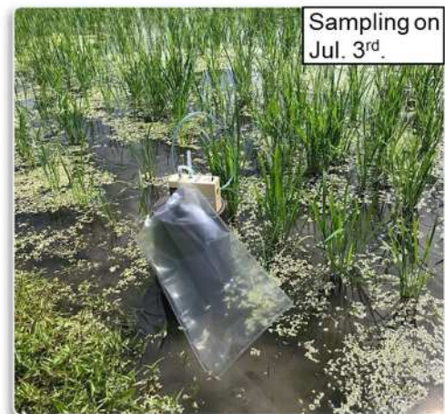
Fig.2 gas sampling by the chamber
