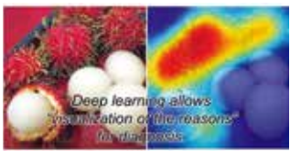
FIG. Diagnosis of "fruit crop species" by ResNet50, and backpropagation of the contributors to the original picture
