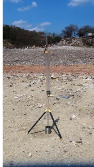
Fig. 7 Constant-head infiltration test using GPI method on the site No.1
